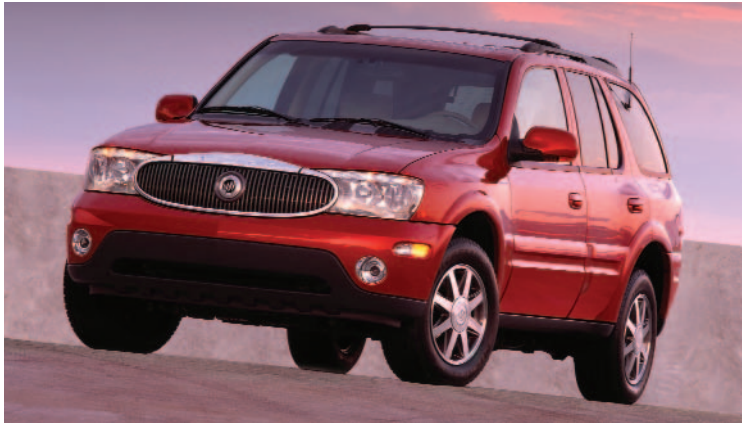
STEEL HEAVY: The Rainier, Buick's first SUV, has around 1,300 pounds of flat-rolled steel, several hundred pounds more than Buick's biggest car, the Park Avenue.
